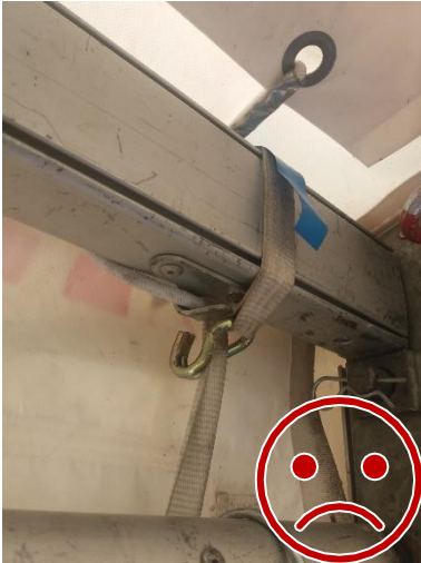
The strap will shear as it tightens.
